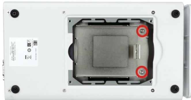
Figure 3-3: HDD Bracket Retention Screws
