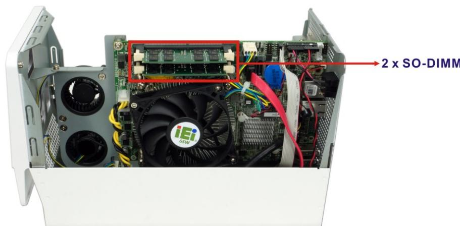
Figure 5-1: SO-DIMM Location
