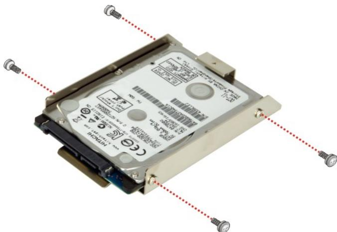
Figure 3-4: Inserting the HDD
