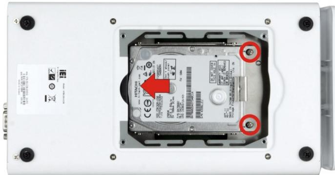
Figure 3-5: Installing the HDD
