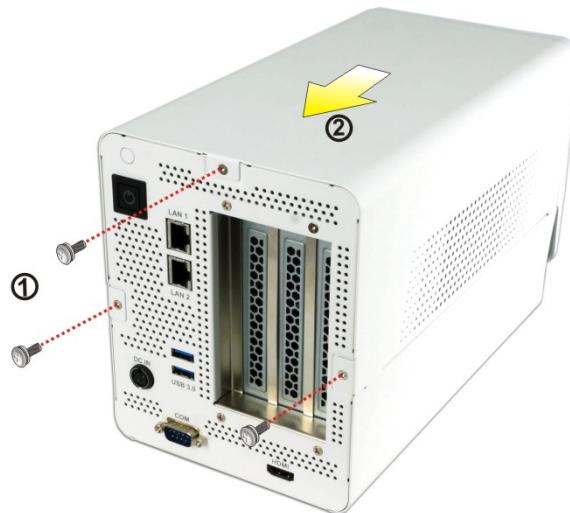
**Figure 3-1: Top Cover Retention Screws**
