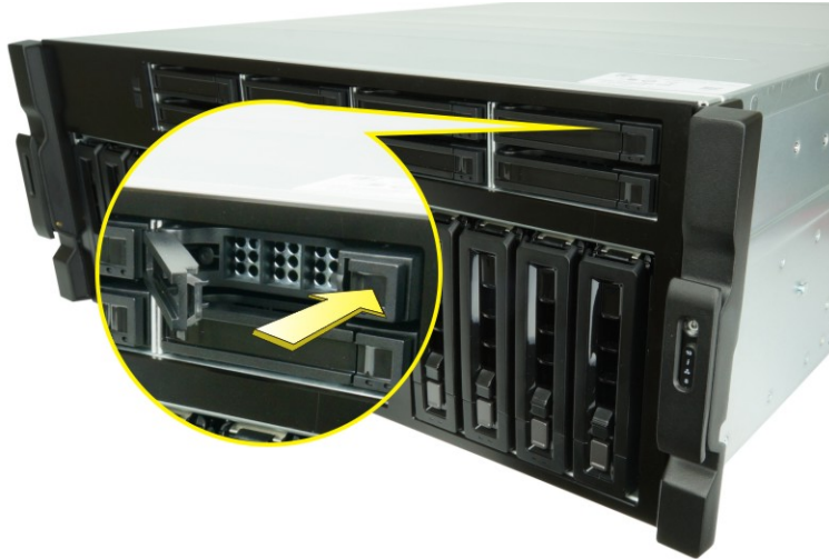
Figure 3-5: Release Drive Tray (2.5")
