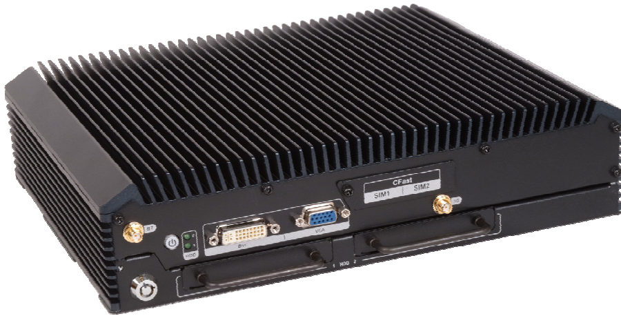
Figure 1-1: IRS-100-ULT3 Railway Surveillance System
