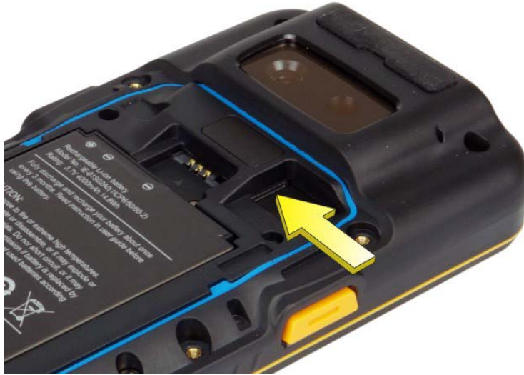
Figure 3-7: microSD Card Slot
