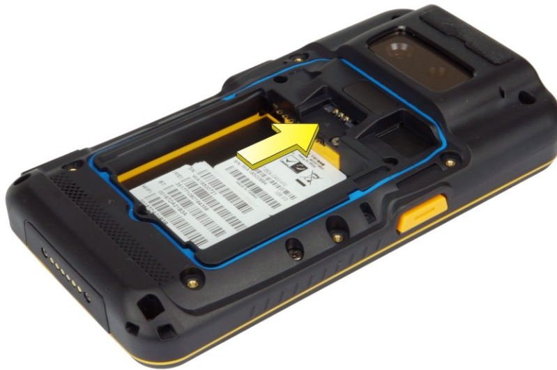
Figure 3-6: SIM Card Installation
