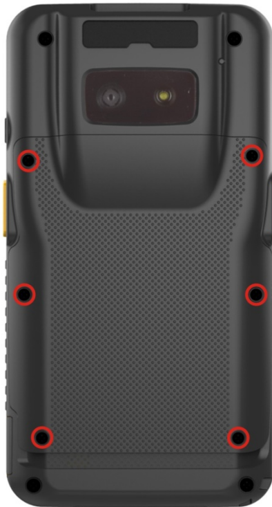
Figure 3-4: Battery Cover Retention Screws
