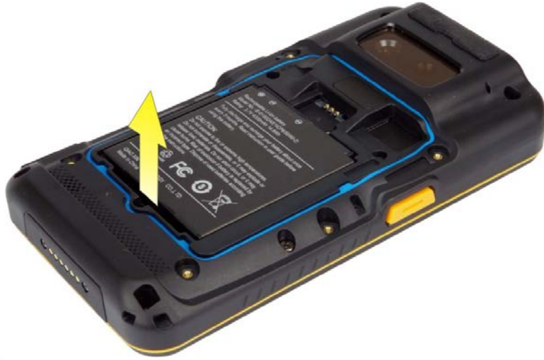
Figure 3-5: Removing the Battery
