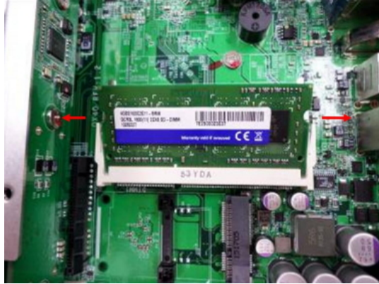
Figure 4-2: Pull the Retention Clips on Each Side
