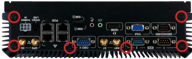
Figure 3-4: Rear Panel Retention Screws
