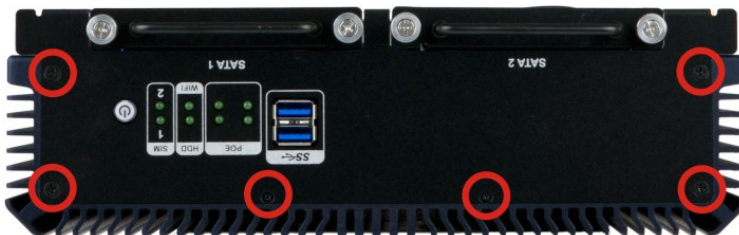
Figure 3-3: Front Panel Retention Screws
