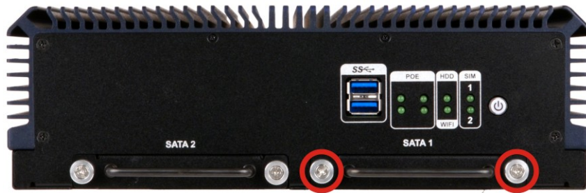
Figure 3-15: SSD Bracket Retention Screws
