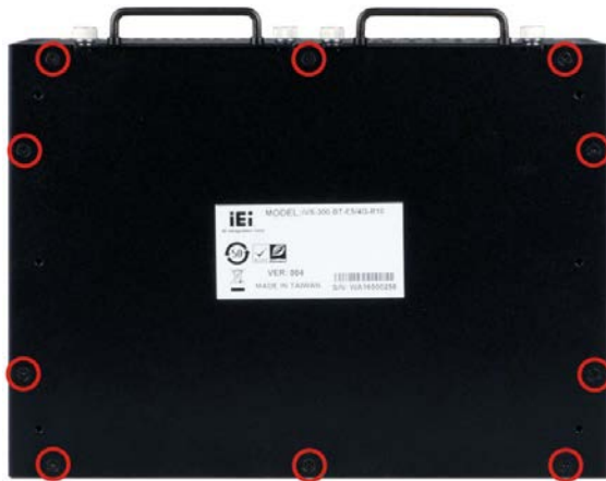
Figure 3-1: Bottom Panel Retention Screws
