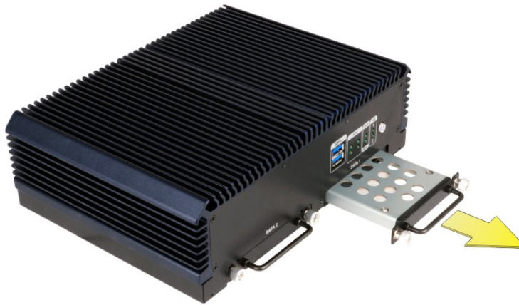
Figure 3-16: Removing SSD Bracket
