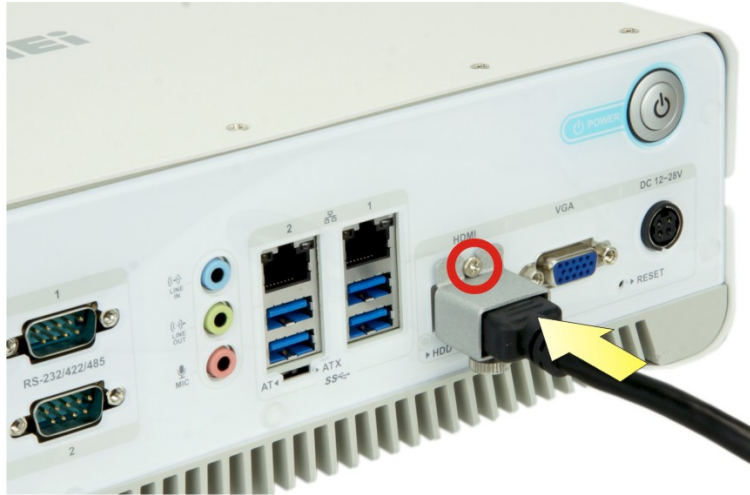
Figure 3-17: Secure the HDMI Cable Holder
