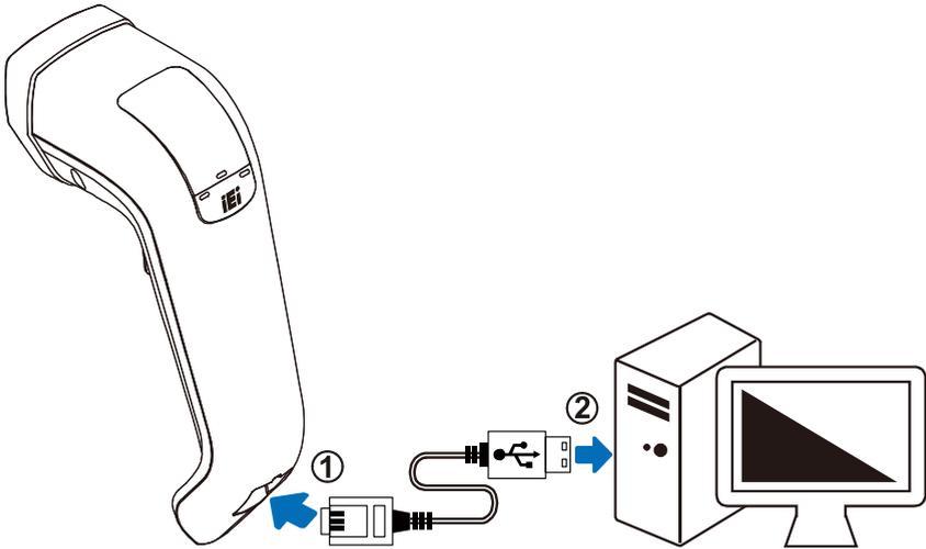
1. Connect the RJ-45 connector of the supplied RJ-45 to USB cable to the RJ-45 port on the HTDB-100F/100FM. Ensure to push the connector to the end until the user hears a “click”.
