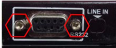
Figure 3-12: Hex Jack Screws for Securing RS-232 Connector
