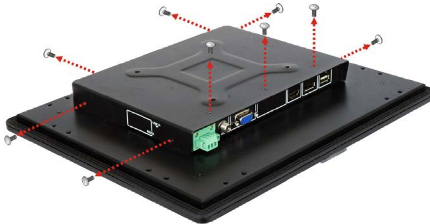
Figure 3-10: Rear Panel Retention Screw Removal (DM-F12A ~ DM-F24A)
