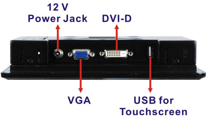
Figure 1-5: Bottom Panel Connectors (DM-F65A/08A)
