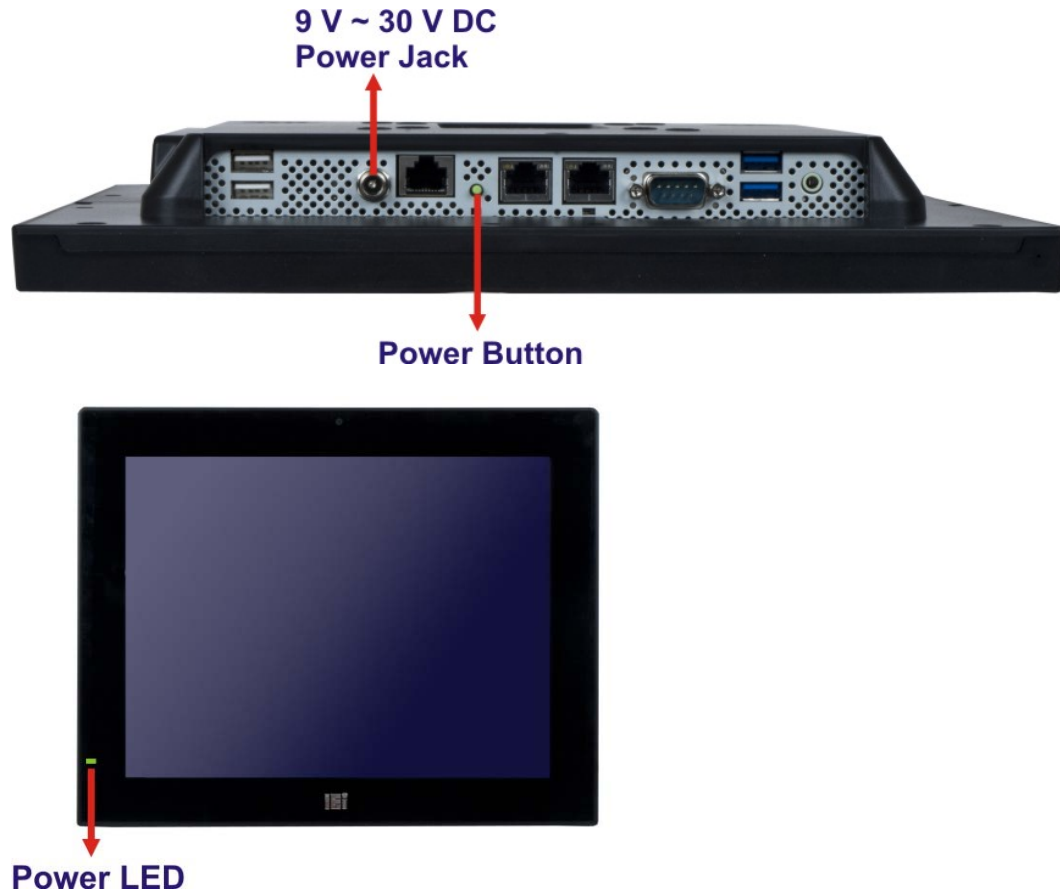
Figure 3-29: Powering On the System
