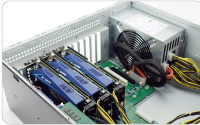
Figure 3-9: Multiple Mustang-200 Installed
