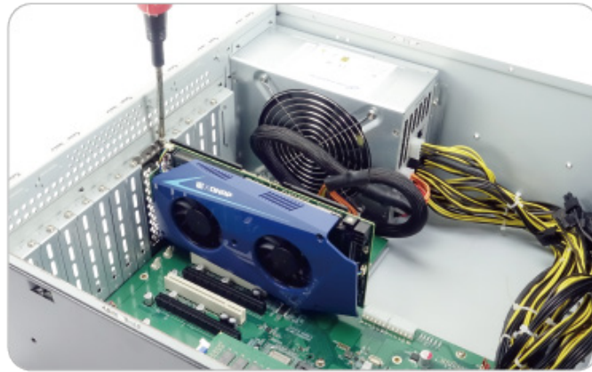
Figure 3-6: Install and Secure Mustang-200
