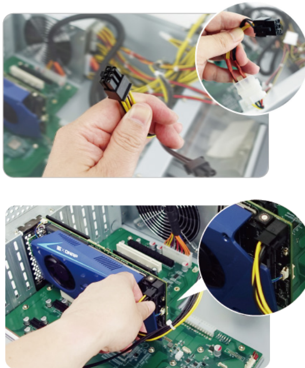
Figure 3-7: Power Cable Connection
