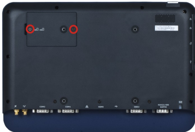
Figure 3-3: SIM Card Slot Access Panel Retention Screws
