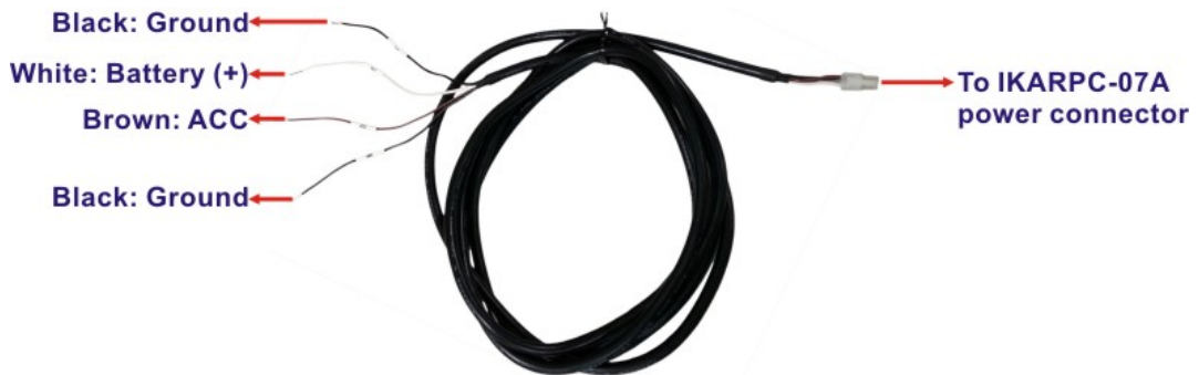
Figure 3-12: ACC Power Cable
