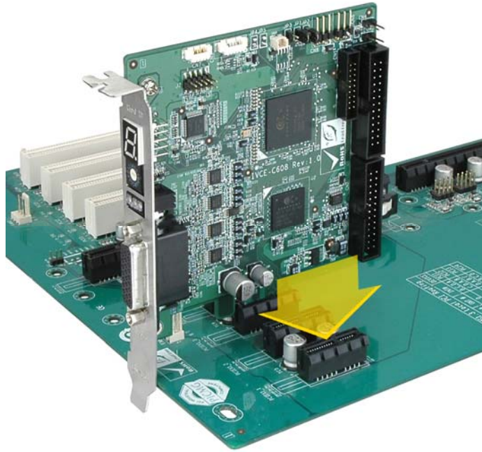
Figure 5-1: IVCE-C608 and IVCE-C604 Installation
