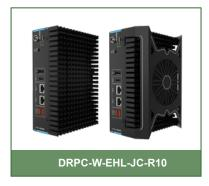
The DRPC-W-EHL-JC-R10 is a compact embedded system and designed for 3.5" single board computers. With the two-dimensional heat conduction and low wind resistance design on the surfaced which means you don't need extra thermal solution to form the heat dissipation part. You can get higher hardness, and benefit from the reduced production cost resulting from shortening manufacturing time .Furthermore, the height of aluminum extrusion can therefore be downsized to make the product light weight.
