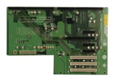
SPE-9S-R11 7-slot PICMG 1.3 backplane with one PCle x16 slot (x8 signal), three PCle x4 slots and three PCl slots (PCle Gen 3.0)
