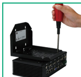
1: Tighten the screws in the rear of the AFOLUX PPC VESA mounting holes
