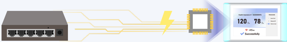
Built-in controller auto-negotiates power with PoE switch
