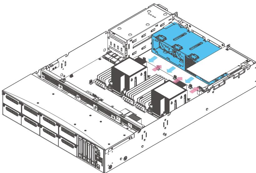
Users can define CPU fan and system fan speed and temperature profile in the BIOS menu. When the system is in idle or running less demanding tasks, smart fan is able to bring down the level of noise produced by rotating fans. The adjustable settings allow the PUZZLE series run with less noise while extending the fan's lifespan, enhancing system stability and durability.
