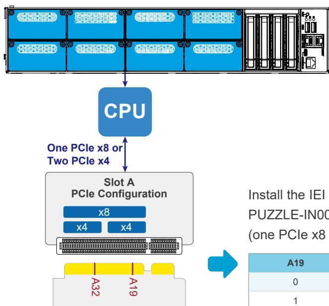
Install the IEI Pu1M-100G2SF-E810 networking module into the slot of the PUZZLE-IN005. All slots support 8 lanes of PCIe gen4 signal from CPU (one PCIe x8 or two PCIe x4).
