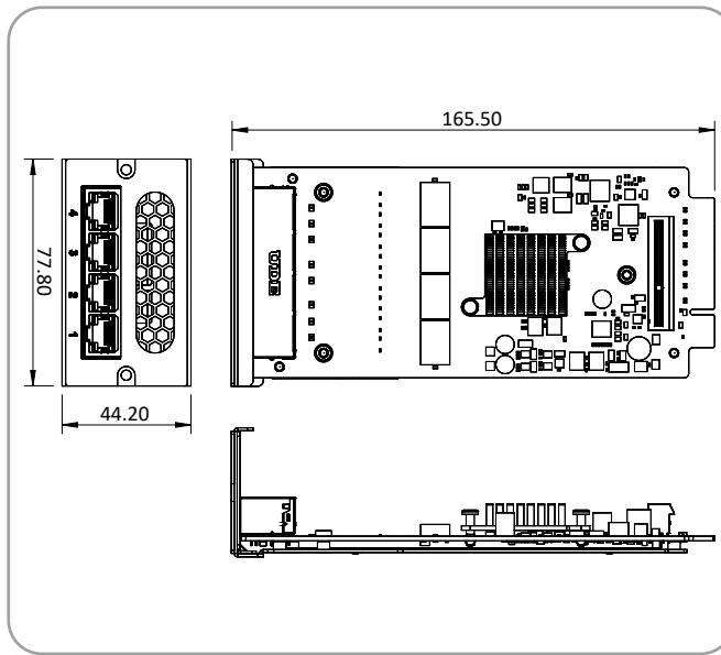
Intel® Ethernet Controller I350-AM4 based Network Interface Card with 4 x RJ45 by 2 PCIe 2.0 x4 interface, RoHS
