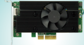
Mustang-V100-MX4 Intel® Movidius™ Myriad™ X MA2485 VPU
