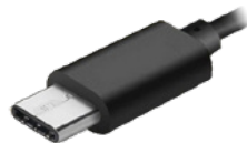
Internal USB 2.0 Type C For debugging by UART
